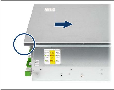
Figure 52: Placing the housing cover
